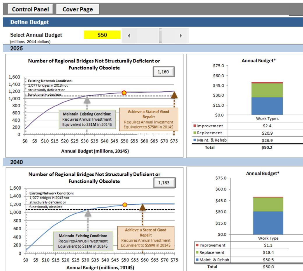
**FIGURE 7. Example of Results from Bridge Asset Management Planning Tool's Performance-Based Condition Assessment**
