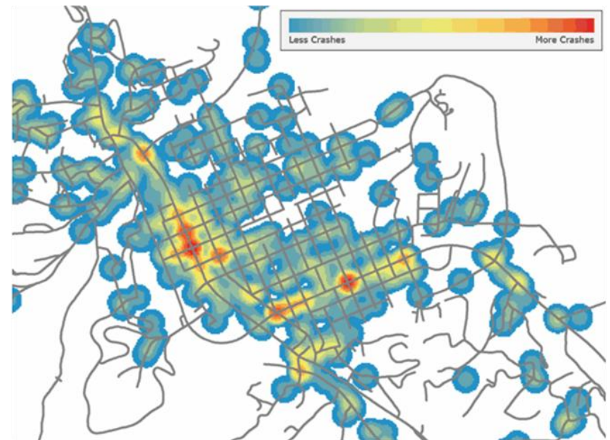
Example: Heat Map – density of crashes per unit area (Network Screening category)
